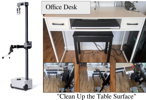
Fig. 13: We trained a Stretch robot on a multi-step task "Clean Up the Table Surface" using URDFormer prediction
