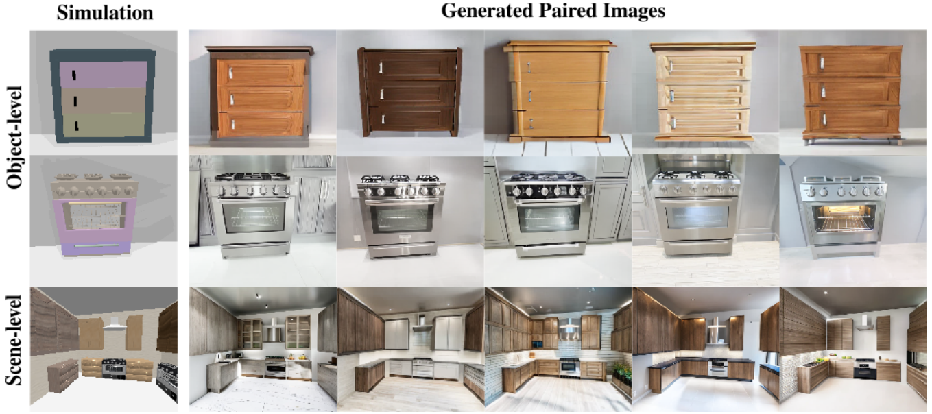
Fig. 3: Controlled Generation: Rendering URDF models in simulation and generating paired images with a guided diffusion model.
